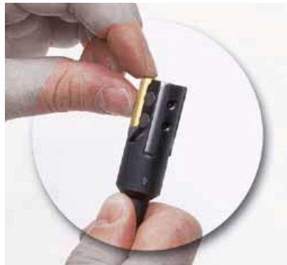
4. Press the insert firmly against the axial limit stop and the positioning balls ⑤.
