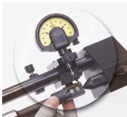
6. Set the gauge on the guide rail lying behind the cutting ③ edge to zero.
