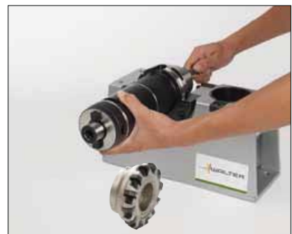
9. Screw the NC tool elements together using the master.
