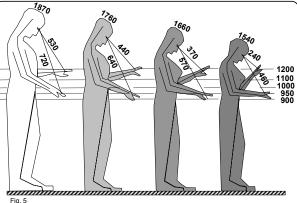
Fig. 5 Visual distances and underarm positions illustrated depending on body height and work height
